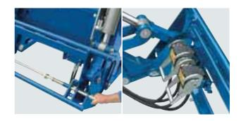
QUICK RELEASE FRAME Mechanical or hydraulic; safe, quick and reliable attachment change. A 3rd and 4th service are available for quick attachment connection.
